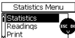
The statistics refers to the whole batch. If the group into blocks option has been disabled (block size: 1), statistics will be calculated from single readings (Single readings statistics).
