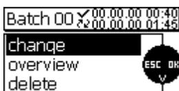
Press function key MENU and select “Database”. Press OK to confirm. The currently active batch is marked by an arrow.
