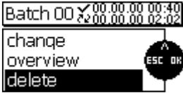
Press function key MENU and select “Database”. Press OK to confirm. Use up/down arrow keys to select the requested batch. Press OK to confirm. Select “delete” and press OK to confirm.
