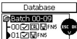
The data base is for management of your batches. You can create new batches, define their calibration methods and parameters as requested or open existing batches to start a measuring series. With the MiniTest 720 and 730 models (featuring 10 batches), all batches are listed in one single list.
