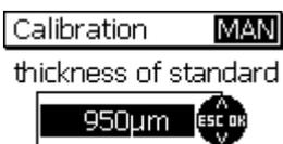
Press OK to confirm the calibration point.
