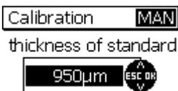
Press OK to store the calibration point. Press OK once again to complete the calibration procedure.
