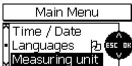
This menu item is for setting the measuring system. You can select metric system (“ $\mu\text{m}$ “, “mm“, “cm“) or imperial (“mils“, “inch“ and “thou“). The measuring units within a measuring system will be automatically set by the gauge according to the thickness being taken.
