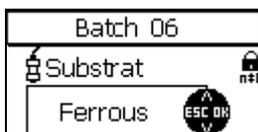
The parameters "calibration method", "substrate", "offset" and "block size" can only be changed as long as there are no readings stored in your batch. As soon as there are readings stored in the batch, a lock symbol will appear on screen to indicate that the requested parameter cannot be changed.
