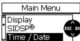
The gauge features a quartz-controlled time clock to indicate date and time. The current time is shown top right in the status line (visible in measuring mode only). The time clock is also used for fixing date and time of creation / last modification of a batch. Date and time of creation/ last modification will also be stored and indicated with a batch and displayed while opening this batch.
