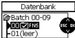
Please note: At initial switch on or after a total reset, the batch # 00 with a preset factory calibration becomes active. It is related to the sensor connected (e.g. FN5). With the MiniTest 740 model, this batch always relates to currently connected sensor. Now you can directly proceed on measurement.
