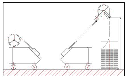
The ECO ARC 350 can be operated with hasp spools decoiling device as well as drum decoiling device.
