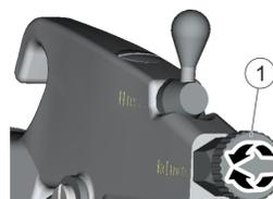
Fig. 9: Adjusting circular jet
