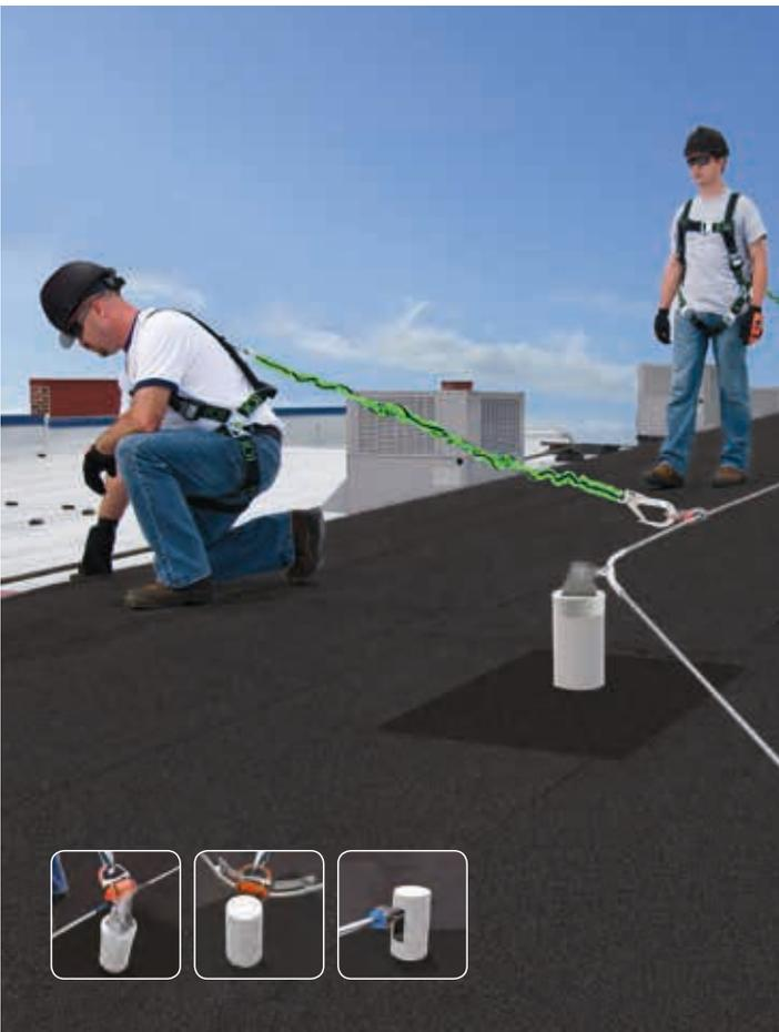
The Söll ShockFusion® horizontal lifeline (HLL) system reduces fall distance (minimised line deflection) while effectively managing system forces to maintain a safe connection to a variety of roof structures. The unique surface-mounted design eliminates the need to penetrate the roof structure, making installation quick and easy while reducing labour costs.
