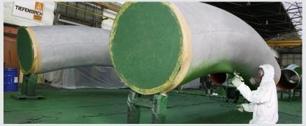
Automatic guns and rotary atomizers for manual and automatic lances Pipes with a diameter of 50-800 mm can be coated internally without turning the pipe using a rotary atomizer. The coating is applied while drawing the movable lance backwards out of the pipe.
