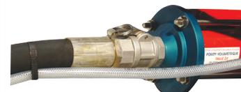
The extension couples onto the pump head.
