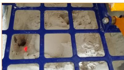
Machine tank level management by laser measuring that allows a minimum of wasted product
